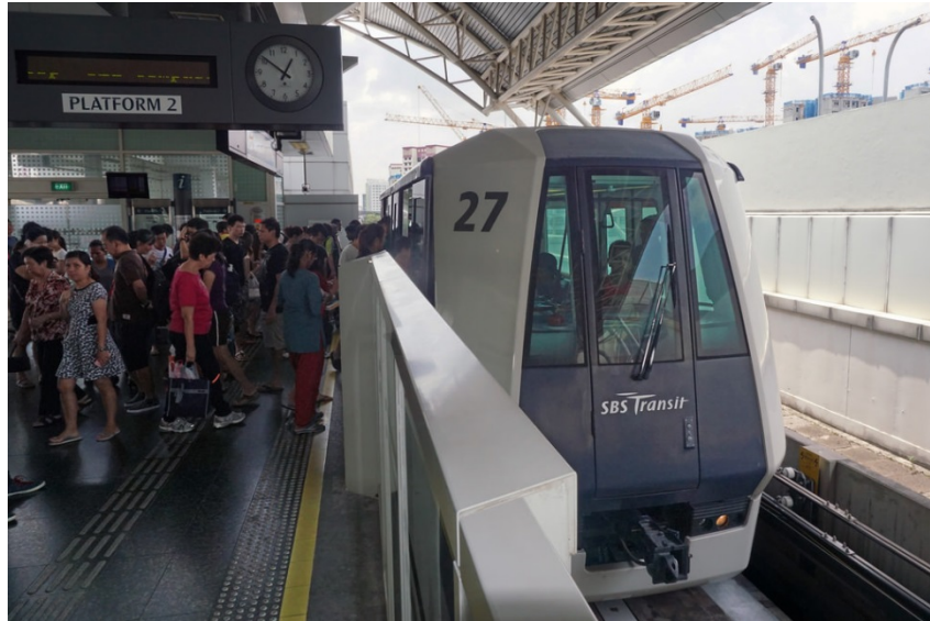
Figure 6-1: Singapore Sengkang LRT Station with Half-height Barrier Wall/Platform Doors, MHI Crystal Mover APM (Image Credit: Peter Velthoen)
