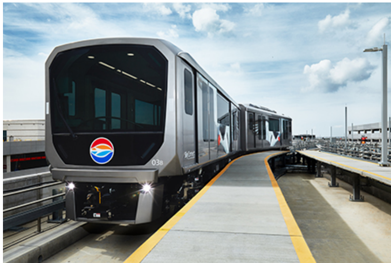
Figure 7-5: APM Emergency Walkway Example, TPA SkyConnect APM (Image source: L+E)
